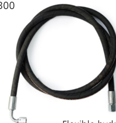
T30-3031 Flexible hydraulique 350 bars R2T5/16 JIC FJ9/16 x FJ9/16 90° L2300
